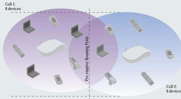
Pre-emptive roaming occurs close to the cell 'edges', ensuring that the load on any given access point is limited to those devices within the actual cell. Users experience higher and more consistent connection speeds, resulting in smoother running of applications.
