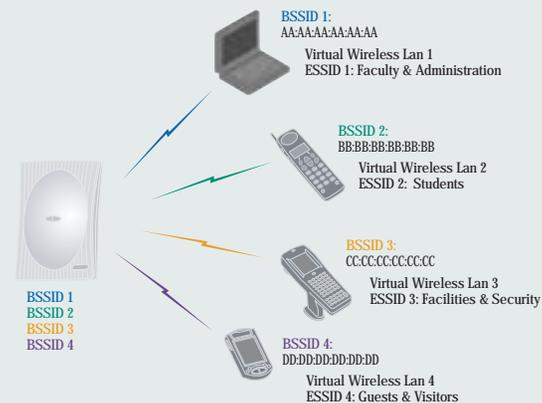
Virtual AP provides support for multiple BSSIDs, enabling the creation of true wireless VLANs. Broadcast traffic is sent only to recipients within a specific wireless VLAN (ESSID), improving overall battery life of client devices and network throughput, and ensuring security and confidentiality for broadcast traffic.
