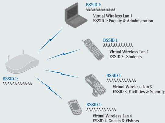
In a typical access point architecture, VLANs are defined using multiple ESSIDs. Since access points support only one BSSID, broadcast traffic intended only for Faculty and Administration (ESSID1) will be sent to all VLANs—Students (ESSID2), Facilities and Security (ESSID3) and Guests and Visitors (ESSID4). The resulting processing of unnecessary messages reduces battery life and network throughput, and delivery of messages to unintended recipients presents security and confidentiality issues.
